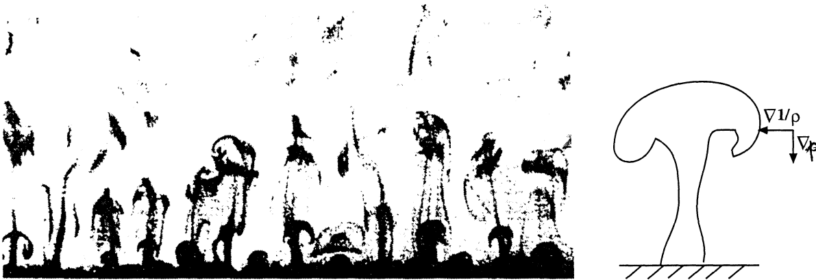
Figure 7. Visualization of 'mushroom' plume vortices rising from a heated plate (from Sparrow et al. [57]).
